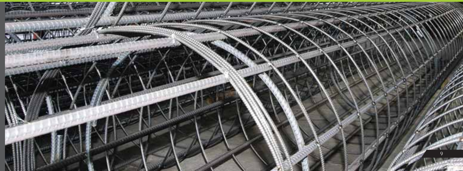
Bored pile cages are used in foundation and contiguous bored piles. The machine-welded bored pile cages ensure consistent quality. These cages can be delivered to the point of use as required and need minimum site labour for installation, thereby increasing construction speed and minimising site material inventory.
