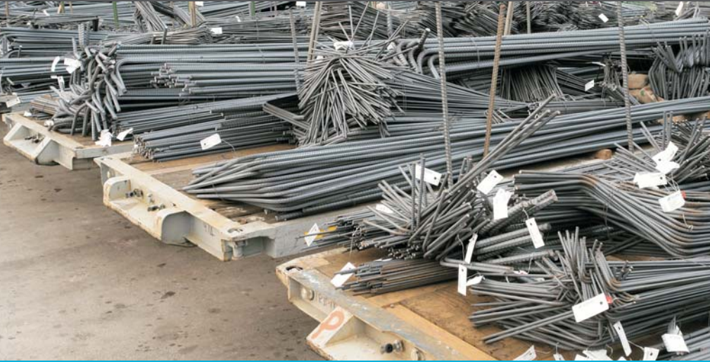
CAB rebars ready for delivery
